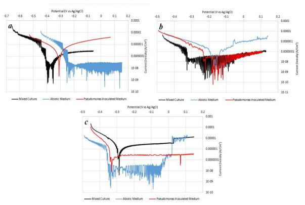
Fig 2. polarization curves of carbon steel immersed in medium with (a) pH=6, (b) pH=7, (c) pH=7.5
